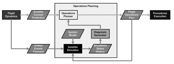
Figure 4 - The operations planning subsystem data flow.
