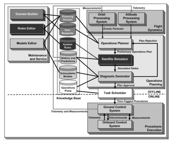
Figure 3 – The new satellite control architecture.
