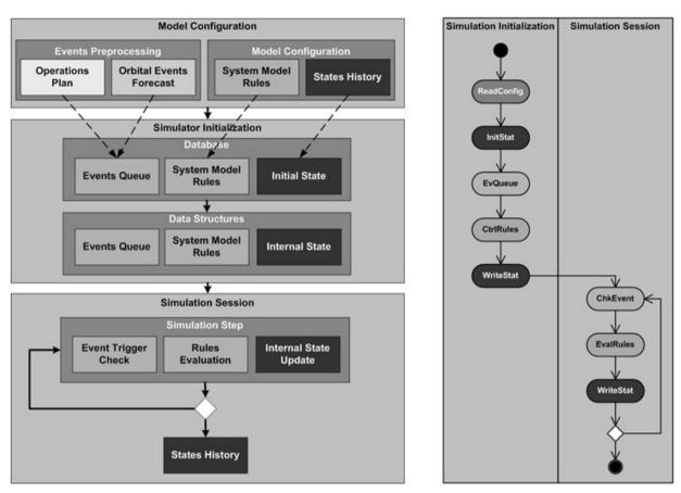
Figure 6 - The satellite simulator working phases and activities diagram.
