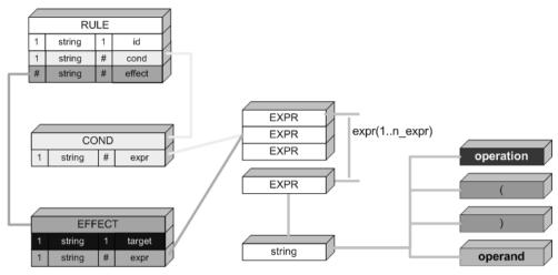
Figure 10 – Simulator rule data structure architecture.
