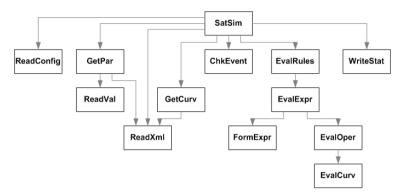
Figure 16 – Hierarchy diagram of the satellite simulator engine.
