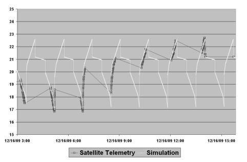
Figure 18 – Example of satellite simulation result (SCD1 battery voltage).
