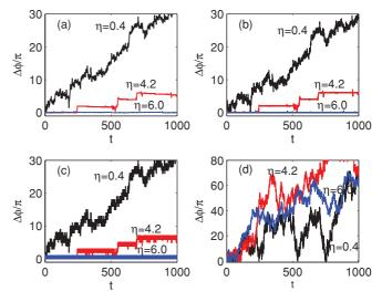
FIG. 7. (Color online) Time evolution of the phase difference of two coupled Lorenz systems for three different coupling values: (a) PEMF method, (b) arctangent on the projection of the attractor, (c) wavelet method with s = 1.0, and (d) wavelet method with s = 2.0.
