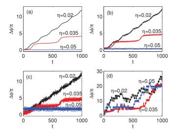
FIG. 3. (Color online) Time evolution of the phase difference of the Rössler oscillators in a phase coherent regime (a = 0.16) for three different intensities of coupling, as indicated, for (a) the PEMF method, (b) the arctangent method, (c) the wavelet method with time scale s = 5.4, and (d) the wavelet method with time scale s = 5.5.
