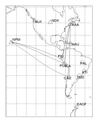
Fig.1 - The receiver bases of the SAVNET array ( $\Delta$ ), transmitters ( $\Diamond$ ) and VLF propagation paths.
