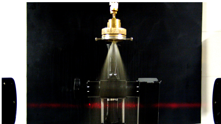
Figure 2. View of the injector with the laser beam emitted from the Spraytec laser system.
