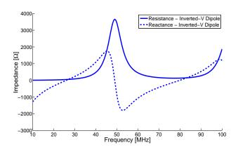
Figure 5: Simulated impedance characteristics for the Inverted-V dipole.
