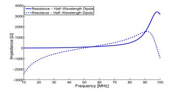
Figure 7: Simulated impedance characteristics for the Half-wavelength dipole.
