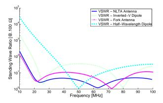
Figure 10: Standing wave ratio at the feed of the antennas NLTA (dark blue), inverted-V (light green), Fork (pink) and Half-wavelength dipole (light blue) to a normalized impedance of  $100\Omega$ .
