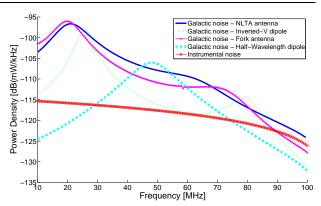
Figure 8: Power density at the receiver input to the antennas NLTA (dark blue), inverted-V dipole (light green), Fork (pink), Half-wavelength dipole (light blue) and instrumental radio noise (red).
