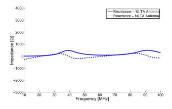
Figure 4: Simulated impedance characteristics for the NLTA antenna.
