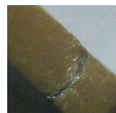
Fig. 9. Flashover channel formed on the capacitor 2 border.
