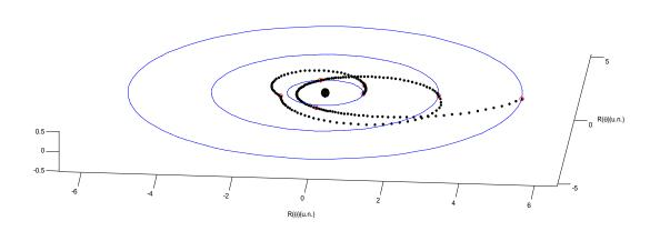
Figure 5. Seven-burn orbit transfers,  $r_0 = 1$  (Earth),  $r_f = 5.202803$  (Jupiter). Solution 1, with 7 burns and  $\Delta V_T = 2.234601$ .
