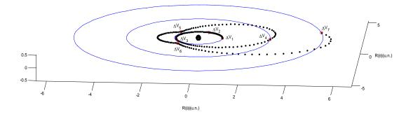
Figure 6. Seven-burn orbit transfers,  $r_0 = 1$  (Earth),  $r_f = 5.202803$  (Jupiter). Solution 2: with 7 burns and  $\Delta V_T = 3.249184$ .
