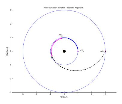
Figure 3. Four-burn orbital rendezvous, simulation 2:  $r_0 = 1$ ,  $r_f = 3$ .
