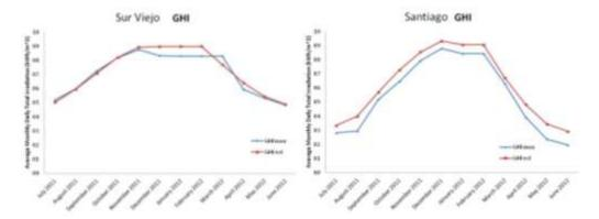
**Figure 6**: Comparisons between satellite estimations and ground measurements for the monthly averages of daily total radiation at Sur Viejo (left) and Santiago (right).
