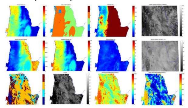
**Figure 4**: Input data for the Chile-SR model (temp and humidity); atmosphere type, GOES images, effective cloud covers and estimated solar radiation for part of the Atacama Desert in Northern Chile. Interesting to note the presence of cloud covers that severely diminish DNI values. Data for April 12 2012 at 16:40 UTC.
