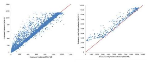
**Figure 7**: Comparisons between satellite estimations and ground measurements considering averages for the complete 2011 year for Santiago. Left: hourly data. Right: daily data.
