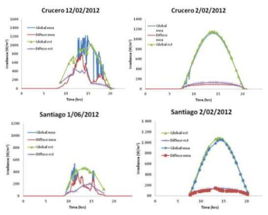
**Figure 5**: Comparisons between satellite estimations and ground measurements for cloudy and clear days at Crucero (23° S) and Santiago.
