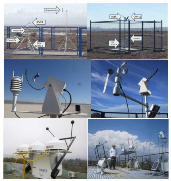
Figure 2: Four different configurations for RSBR stations (From top left to bottom right: Coya Sur, Sur Viejo, Pozo Almonte and Marimaura); one station with tracker, pyrheliometer and ventilation units for pyranometers (bottom left, at Talca); and author Alberto Ortega enjoying himself at the UC Solar Evaluation Lab in Santiago (bottom right) where both BSRN-standard and RSBR radiometers are tested prior to field deployment. Nice vertical development clouds over the Andes Mountains at the back.
