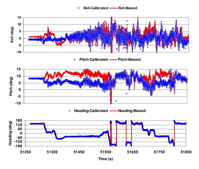
Figure 5 – Attitude angles computed from calibrated and uncalibrated sensors
