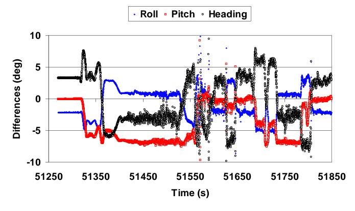
Figure 6 – Differences between calibrated and uncalibrated attitude angles
