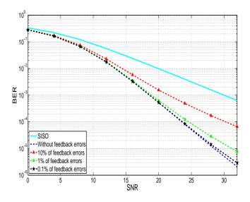
Fig. 5. BER of the proposed scheme with no ideal feedback channel.
