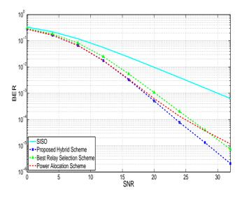
Fig. 2. BER performance for the three relay selection schemes.
