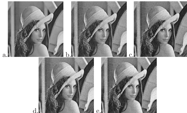
Figure 3: Generalization tests with Lenna image: a) original image; b) Gaussian degraded with 1% noise; c) restored image by a 3x3 Wiener filter; d) ANN result - multiscale approach, 80% similarity; and e) ANN result - multiscale approach, 90% similarity.
