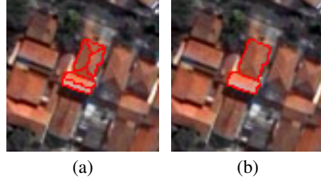
Figure 6: Objects merging process: a) Connected regions, b) re-segmentation taking into account the rectangular shaped regions.
