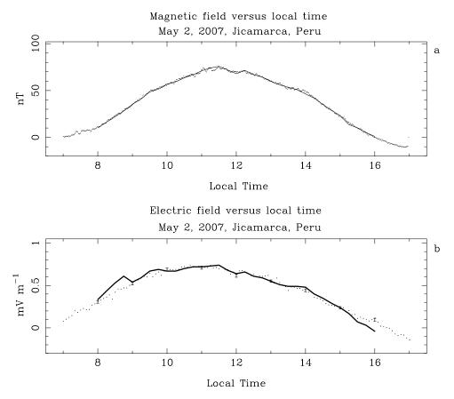
**Figure 1.** (a) Measured (dots) and modeled (solid line) horizontal magnetic field perturbations in the Peruvian sector over Jicamarca (2 May 2007). (b) Measured (dots) and calculated (thick solid line) zonal electric fields over Jicamarca, Perú. The error bars of zonal electric field measurements are also shown.
