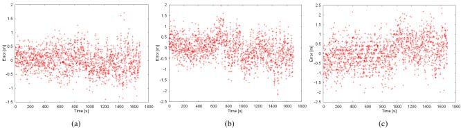
Figure 1: Error components using LSAST method for static data: (a) south; (b) east; (c) vertical.
