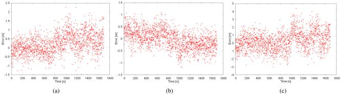
Figure 2: Error components using LAMBDA method for static data: (a) south; (b) east; (c) vertical.
