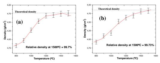
Fig. 4. Density vs. sintering temperature for Ti-10Nb (a) and Ti-15Nb (b). Dotted line indicates the alloy theoretical density.
