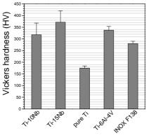
Fig. 5. Vickers hardness values for Ti-10Nb, Ti-15Nb, pure Ti, Ti6Al4V and INOX F138.
