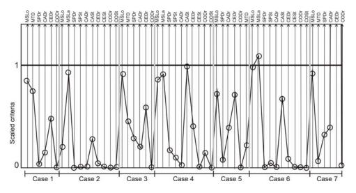
Fig. 5. Normalized criteria in parallel co-ordinates compared with metrics computed for initial solution. Solid horizontal line represent initial performance of the system. Cases: 1) Driving straight ahead over the plane; 2) with Ackermann steering over the plane; 3) straight ahead on a  $20^{\circ}$  incline; 4) equal steering on a  $20^{\circ}$  incline; 5) case 1 in low-traction terrain; 6) case 2 in low traction terrain; 7) case 3 in low-traction terrain.
