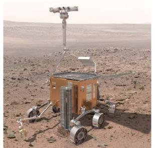
Fig. 1. Artist's view of the ExoMars rover [1] for future planetary mission to Mars scheduled for launch in January 2018; total mass including scientific instrumentation is 250kg; 6 wheels, each wheel actuated for driving and steering (courtesy: ESA).
