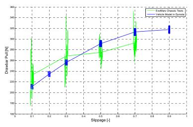
Fig. 3. Drawbar pull as a function of slippage for Mars soil simulant DLR-D2, experimental data taken from [1].
