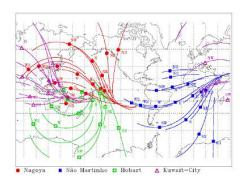
**Fig. 3**: The complete coverage of the GMDN - Global Muon Detector Network with the directions for each MMD?s: Nagoya, Japan 17 directions; Hobart, Australia 13; Kuwait, Kuwai 13; So Martinho da Serra, RS, Brazil 17 (V, N, S, E, W, NE, NW, SE, SW, N2, S2, E2, W2, N3, S3, E3, W3).
