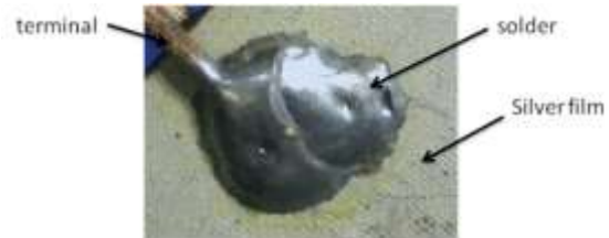
Figure 7. Cooper terminal firmly soldered to the PZT metallic electrode with no cracks or film release.
