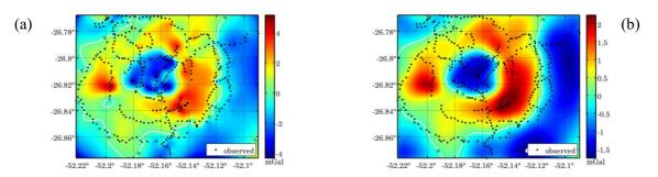
*Figure 2 Residual Bouguer anomaly. (a) at surface level; (b) upward continued to 500 m.*
