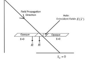
Fig. 4 - The geometry for the calculation of the field due to a canopy simulated by an opaque screen with a square hole.  $\vec{x}_{G}$  is the location on the ground at which the field is calculated, shown at the origin in the Figure.  $\vec{x}_{T}$  is the position of the transmitter,  $\hat{n}$  is the surface normal, and  $E(\vec{x}')$  is the field in the hole.
