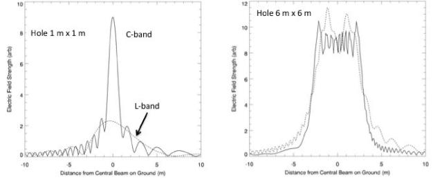
Fig. 5 – The calculated electric field strength at L- (dotted) and C-band (solid) as a function of distance from the central beam on the ground for a 1 m x 1 m square hole and one 6 m x 6 m, not considering the increased attenuation at C-band relative to L-band to water absorption.
