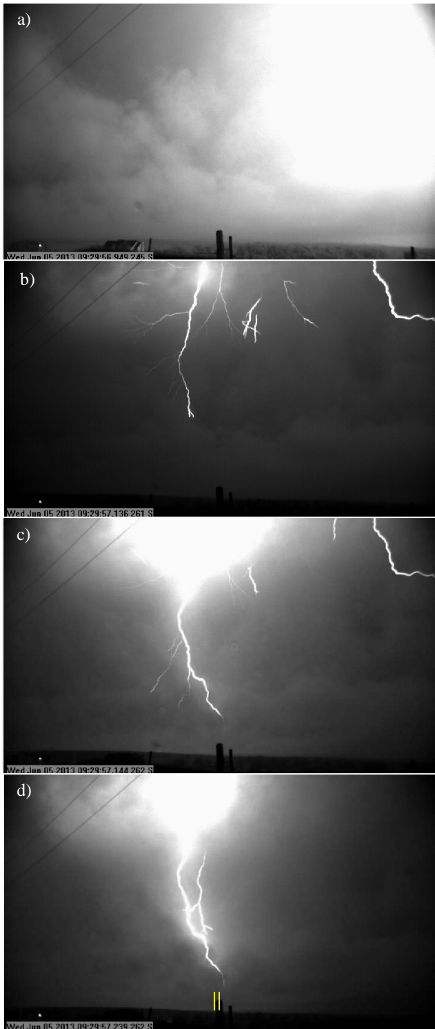
Fig. 15. Video frames from the 2-turbine flash on June 5, recorded by the Miro 4 camera recording at 1000 fps. (a) diffuse illumination from earlier +CG stroke ~50 km south-southwest of the camera location; (b) image of downward propagation positive leader about 8 ms before the +81 kA return stroke that struck the turbines; (c) just prior to +81 kA return stroke; (d) 95 ms after the return stroke. Yellow bars represent turbines that had SCADA reports.
