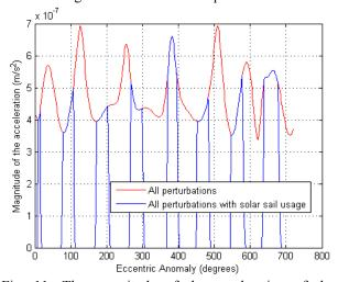
Fig. 11: The magnitude of the acceleration of the disturbing forces for two orbital periods.
