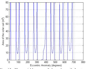
Fig. 13: The variable area of the solar sail for two orbital periods.
