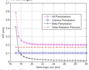
Fig. 5: The KPI values as the semi-major axis increases (17-30 km range).
