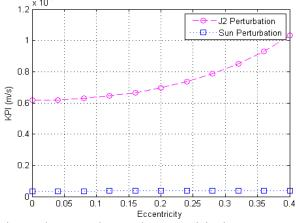
Fig. 7: The KPI values as the eccentricity increases.
