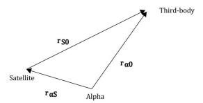
Fig. 2: Illustration of the third-body perturbation formulation.
