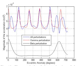
Fig. 10: The magnitude of the acceleration of the disturbing forces for two orbital periods.
