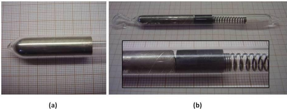
Fig. 2. (a) Growth ampoule for the vertical Bridgman (VB); (b) growth ampoule for the inverted vertical Bridgman (IVB) with an internal spring and a plug to hold the melt in the upside down position.
