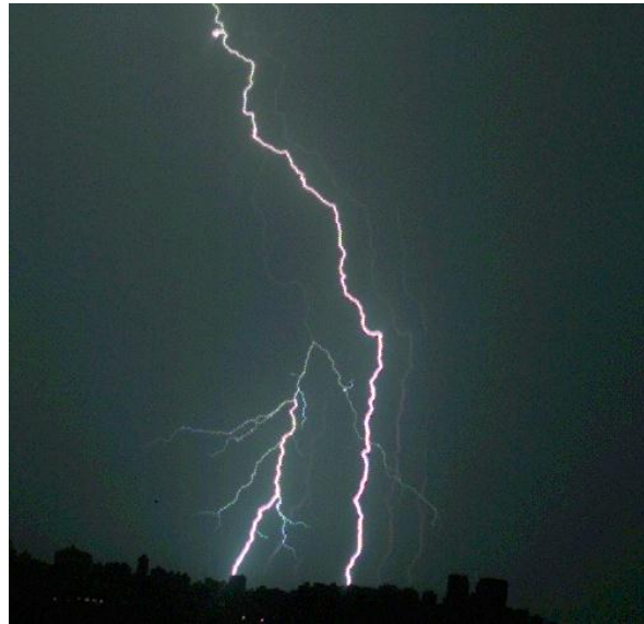
Figure 14 Cropped high-speed video frame of a MGCS event classified as an UI stroke. The left-hand side branch corresponds to the UI process, as the non-uniform brightening suggests. Although there is still visible (although dim) luminosity in the upper part of the channel, its lower region is considerably brighter.
