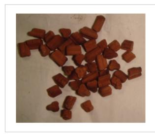
Figure 1. Rh<sub>2</sub>O<sub>3</sub>/Al<sub>2</sub>O<sub>3</sub> catalyst.
