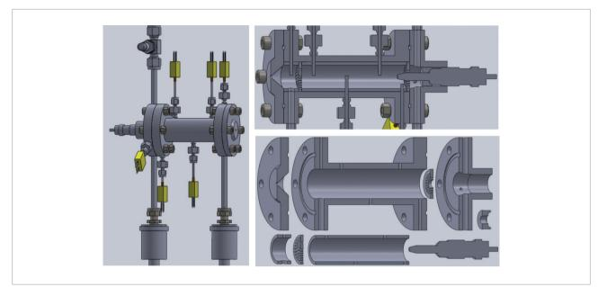
Figure 2. 3D drawings of the thruster with instrumentation and cut views.
