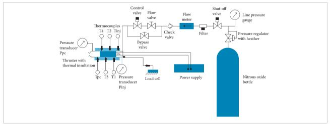
Figure 4. Test bench scheme.
