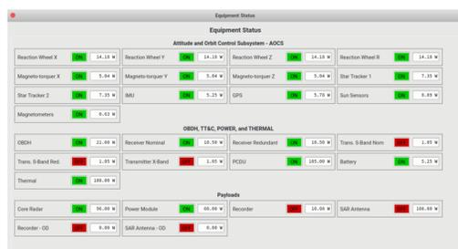
Figure 2: Equipment Module GUI [1]
