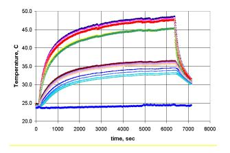
Fig.9. Dry-out under unfavorable inclination of -2 degree 15 W.
