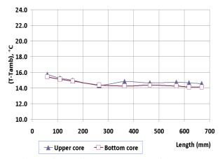
Fig. 5. High equivalent conductance of the HP under unfavorable inclination of -2 degree and 15W.
