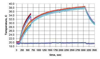
Fig. 7. Start-up with overshoot and delay of 630 sec; heat load is 20W, inclination is +2.5 deg..
