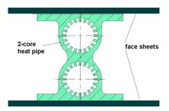
Fig. 1. Two-core heat pipe inserted into honeycomb panel
