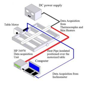
Fig. 2. Experimental setup.
