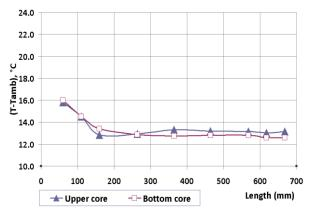
Fig.4. Distortion of the temperature profile under favorable inclination of +2 degrees and heating power of 15 W (trapped slug).
