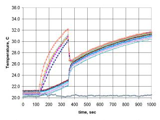
Fig. 10. Temperature overshoot during start-up of the heat pipe at vertical position (15W, 90 deg).
