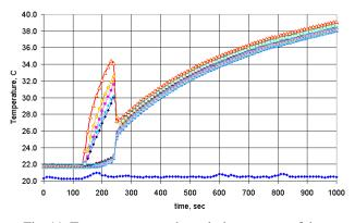
Fig. 11. Temperature overshoot during start-up of the HP at vertical position (25W, 90 deg).
