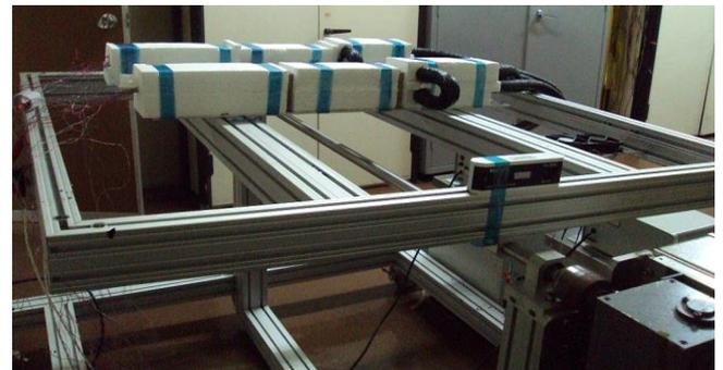
Fig. 17. Both heat pipes installed on the table.
