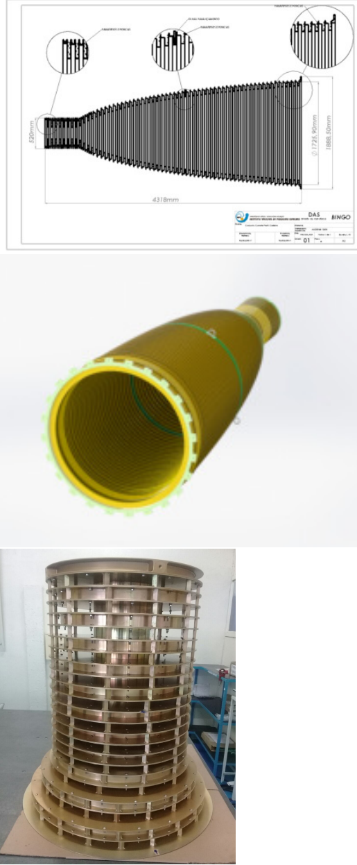
FIGURE 4. Top: Horn blueprint, with details on the corrugation. Center: Horn front view, green rings are machined and contain sockets for suspension rings. Bottom: Throat of the horn already assembled and coated with alodyne.
