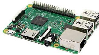
Fig. 12. *Raspberry pi 3, modelo B*
