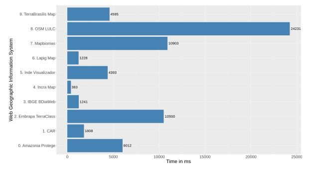
Figure 13. Web Application Load Test.
