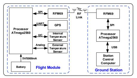
Figure 4: Block Diagram of the RaioSat – Prototype.
