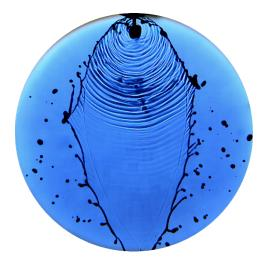
Figure 1. Hidrous ethanol liquid sheet,  $2\theta = 90^{\circ}$ , u = 3.5 m/s
