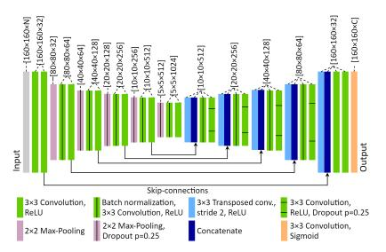
**Fig. 4** Modified U-net architecture (adapted from Ref. 28). The N, in the input size, is the number of bands, while the C, in the output size, corresponds to the number of classes.
